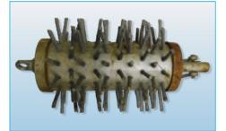
Scraping is a mechanical process in which a device is pushed or pulled through a pipeline to remove built-up deposits on the pipe wall. Because scraping cleans a pipe down to bare metal, this process should always be accompanied by a pipe lining method to prevent accelerated corrosion.
