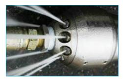
Jetting is the process of using a high-pressured flow of water to scour the interior surface of a pipe to remove scale or other debris that's built up over time.
